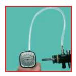
Manual leak test on flexible endoscope
