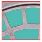
Filter holder with corrosion in the form of particulate
