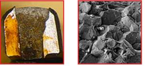
Stress corrosion cracking usually leads to visible cracks and fractures. In some cases, crack formation is not visible because its origin is hidden by
