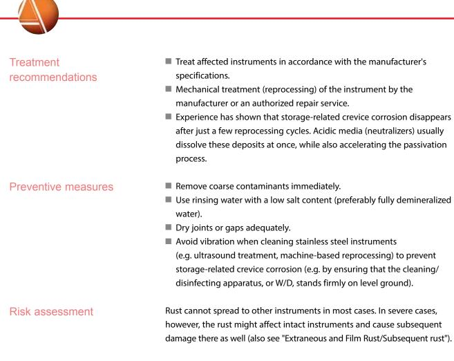
With storage-related crevice corrosion, experience has shown that there is no danger to the affected instruments or to unaffected instruments, because the minor deposit volume is not sufficient to cause damage, unless the phenomenon cannot be eliminated by further reprocessing using acidic media.
