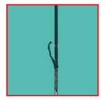
Damaged insulation on HF instrument
