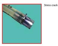
Stress-crack corrosion, e.g. in polysulphone, leads to visible cracks or fractures.
