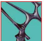
Retractors with discolored black shaft in hardened Cr-steel with the handle and blade remaining bright, made from non-hardenable CrNI steel.
