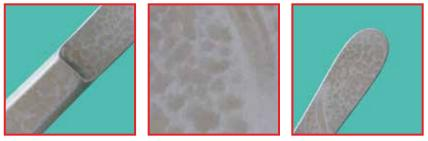
Typical silicate discoloration occurs, <u>regardless of the nature of the surface</u>, over large surfaces, yellow-brown to blue-violet in the cleaning & disinfection process, or in spots, droplet-shaped with pronounced condensation stain-like appearance during the steam sterilization process.
