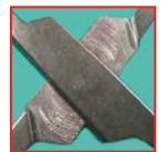
Corrosion due to insufficient use of care products
