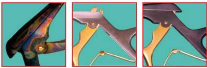
Example: black, TiAIN coated punch. The partial erosion of the layer has caused bright, colorful discoloration or complete removal of the layer with undamaged gold-plated components. Right Punch: as new
