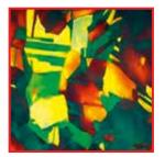
Color etching - austenitic microstructure on rust and acid-resistant instrument steel (500x magnification)
