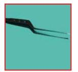
Deformation caused by improper handling
