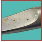
Chloride-induced pitting on instrument.
