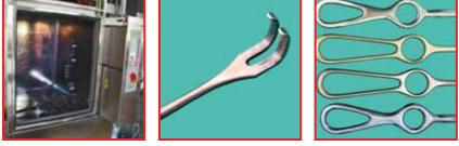
Titanium oxide discoloration occurs mostly on <u>reflective surfaces</u> over large surfaces, yellow-brown to blue-violet, sometimes with a shimmering appearance, in the wash chamber or over the entire surface of the instrument during machine-cleaning.
